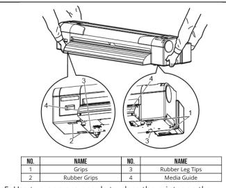
Use two or more people to place the printer on the assembled stand. DO NOT TRY LIFTING THE PRINTER ALONE.
