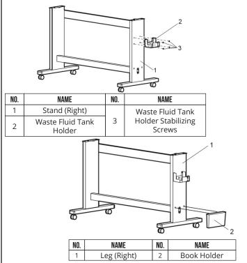
4. Attach the waste fluid tank holder to the upper right side of the stand and the book holder to the lower right side of the stand.
