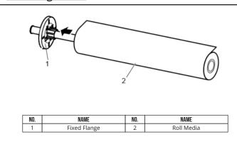
1. Install rolled media onto steel rod scroller so that fixed flange is to the left and movable flang is to the roll's right side when roll feeds from over the top.
