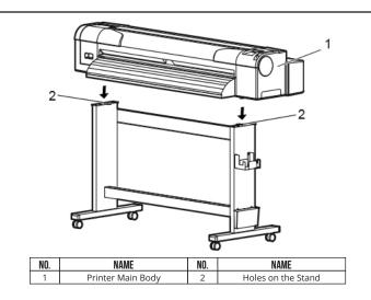
6. Place the product on the stand so that the rear rubber leg tips fit into the holes on the stand.
