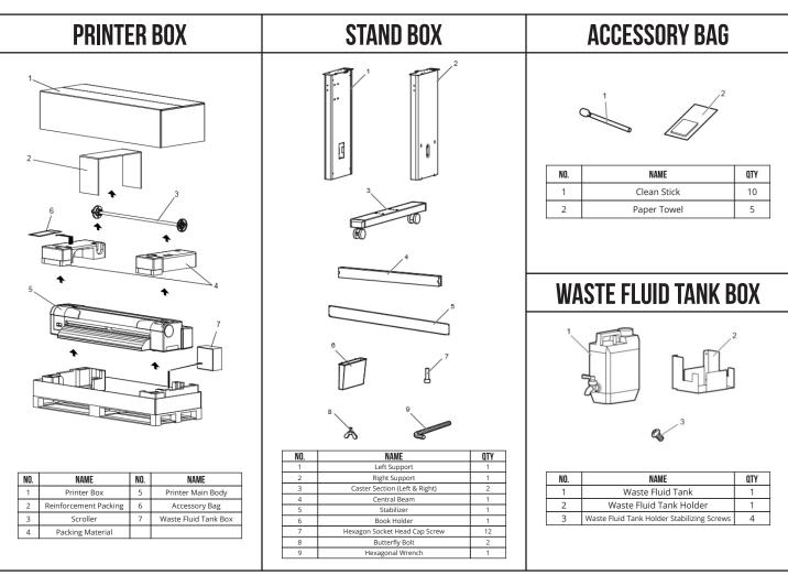
Once all parts are accounted for, follow the instructions and illustrations for assembling the tand and placing the printer. Use two or more people to place the printer on the assembled stand.
