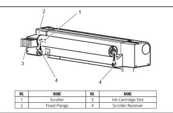
2. Set the scroller onto the scroll receiver with the fixed flange side facing the ink cartridge slots.
